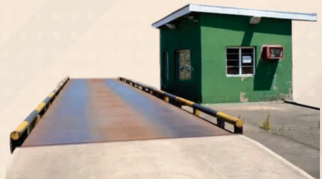
Weigh Bridge Container
